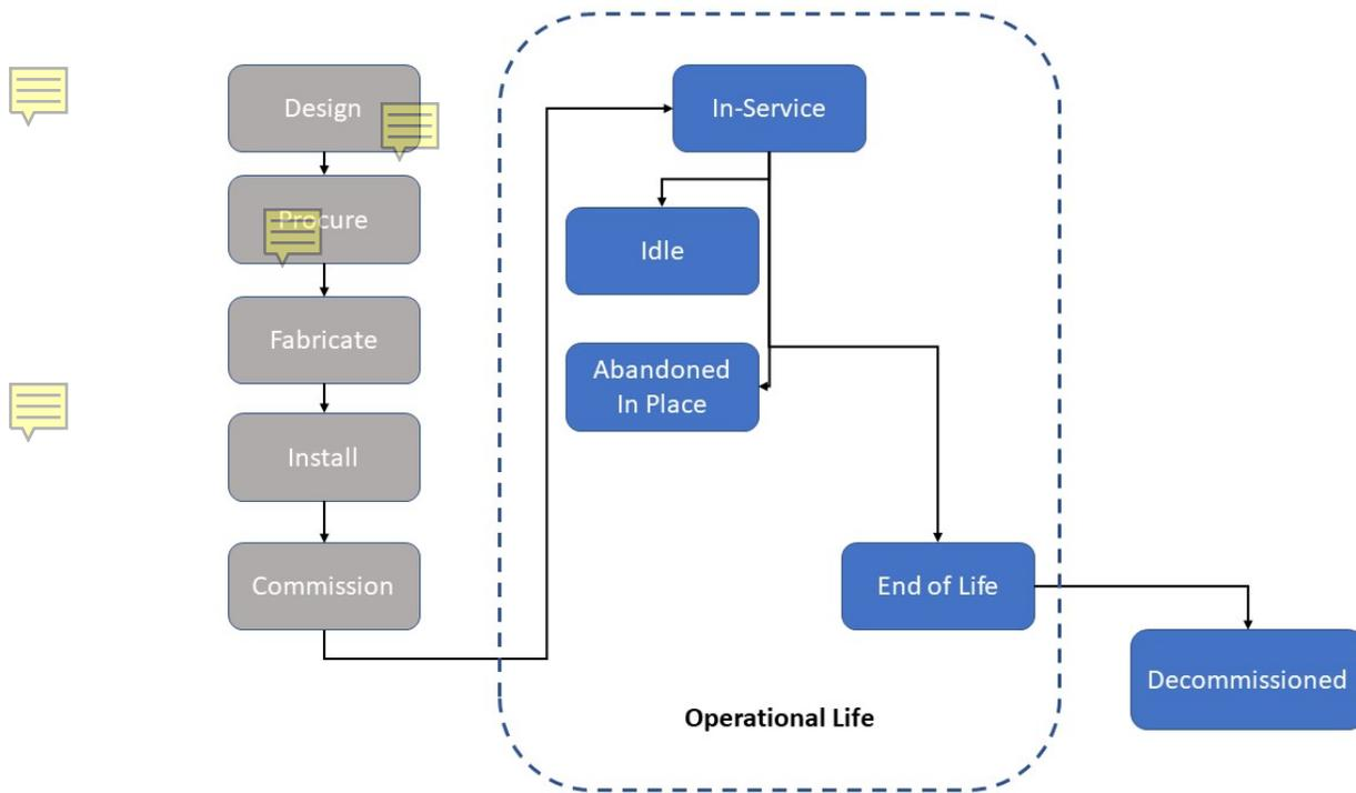
**Figure 2 Lifecycle of Piping Systems**
